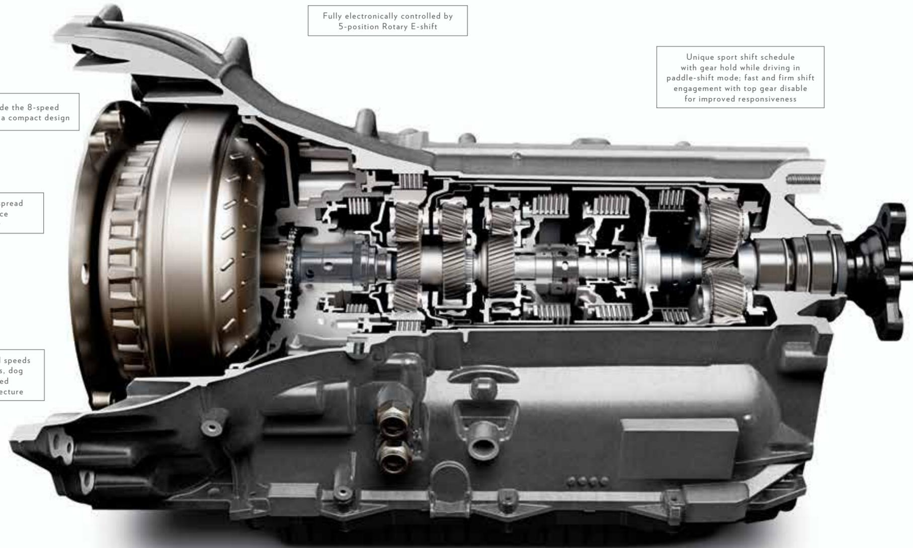
Gearsets are nested inside the 8-speed automatic transmission for a compact design
