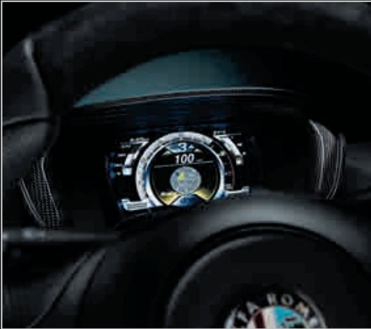
Full-digital instrument cluster with Thin Film Transistor (TFT) display and carbon fibre cluster surround
